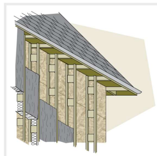
Figure 7-10 Trusses can be hung from the rafters and nailed to the existing wall
