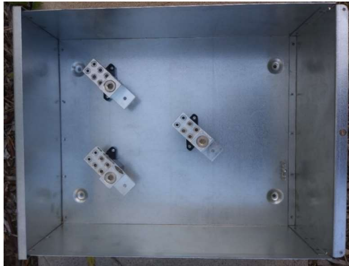
Photo: APS-400 400 ampere Splitter box with 3 connection points for incoming wires and additional lugs to split the service into multiple outgoing feed.
